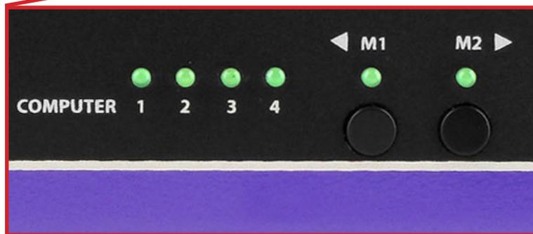
The DPN-4Duo features easy methods of control & switching, including simple front panel buttons and LED indicators for managing KVM control of any four connected computers.
